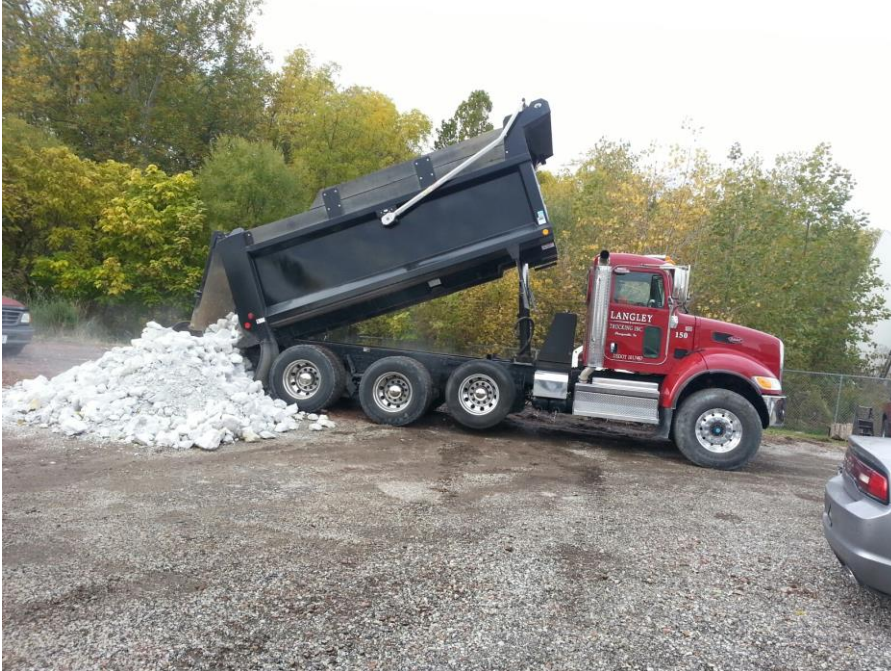
Look October 23rd 2019 at tandem truck with tag wheels delivering stone rip-rap to site
